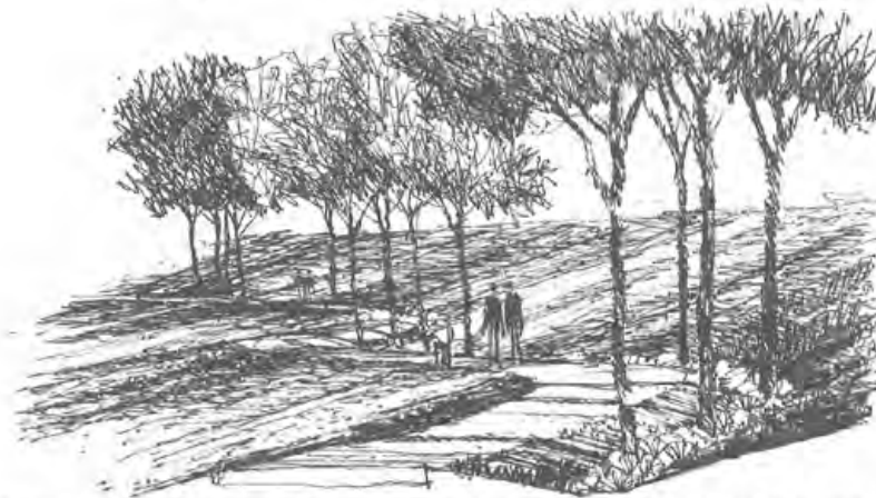
Drainage Corridor Illustration: A network of drainage corridors will connect developed neighborhoods to Westerly Creek and other primary drainageways, serving to detain water and clean pollutants from the urban runoff. As stormwater infiltrates along the canal, it will sustain a network of trees and vegetation. A pedestrian path will allow access for periodic maintenance and cleaning.
